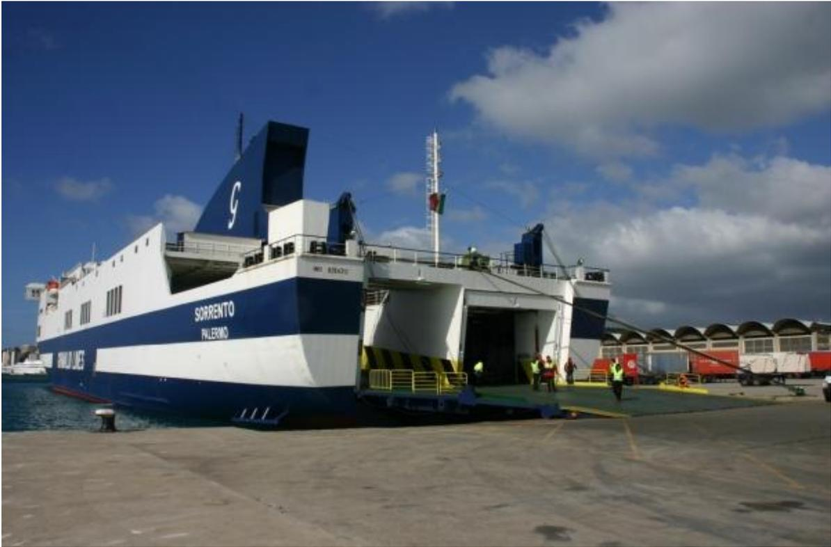
Figure 5. Sorrento stern view. The loading ramp and the two entrances to car deck No 3 (starboard) and to car deck No 4 (port).
