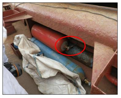
**Figure 13:** The two oxygen (blue) and one propane (red) cylinder that were carried from the Carpenter's Shop to the open deck, after the fire extinguishing operation. The flexible pipe that was connected to the cylinder before it was cut in order to remove it is marked.
