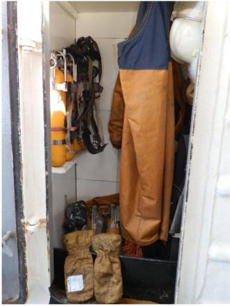
Figure 20: The fireman's outfit stored in the fire locker at the port side of the Accommodation.
