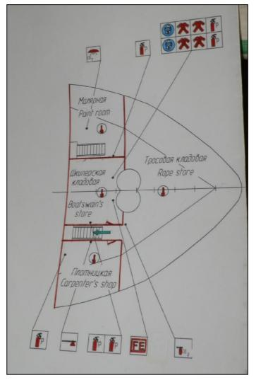
Figure 9: The forecastle area as presented by the vessel's Fire Control Plan (No 53025)
