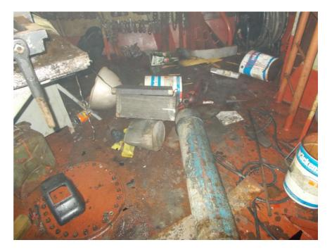
**Figure 16:** The Rope Store as found after the explosion. On the left upper corner of the picture the working bench is shown, while an oxygen cylinder connected to the flexible pipe of the flame tool lies on the floor.
