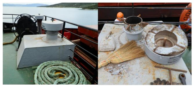
Figure 18: Photos of the ventilation mushrooms placed on top of forecastle's spaces (one port and one starboard side).
