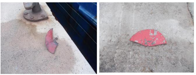
Figure 7: Metal pieces found overboard, casted by the explosion
