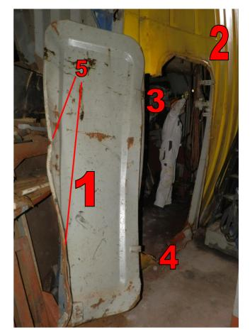
**Figure 14:** The door of the Carpenter's Shop (1) and the internal bulkhead (2). They were evidently deformed, while there were cracks on the door's casing (3) and (4). The paint coating was clear and in good condition. The deep corroded points on the door (5) and at the lower casing (4) cannot be attributed to the oxidation from extinguishing water sprays suggesting that the occurrence had happened quite some time ago.
