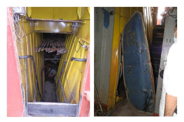
Figure 15: The door and the Starboard bulkhead of the Carpenter's Shop, clearly deformed, yet thoroughly painted.
